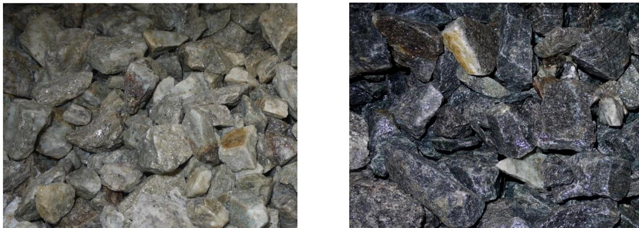
**Figure 3:** Sorting of -70 + 25 mm AHP. Lithium bearing pegmatite product (left) and amphibolite reject (right)
